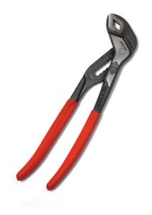
Features & Benefits  $\sim$  Special alloy drop forged steel, hardened for exceptional strength & durability  $\sim$  Slim, long jaws for confined spaces  $\sim$  Box joint design for extra stability  $\sim$  Adjustment positions: 9  $\sim$  Maximal useable jaw capacity: 58 mm Ø  $\sim$  Total length: 300 mm
